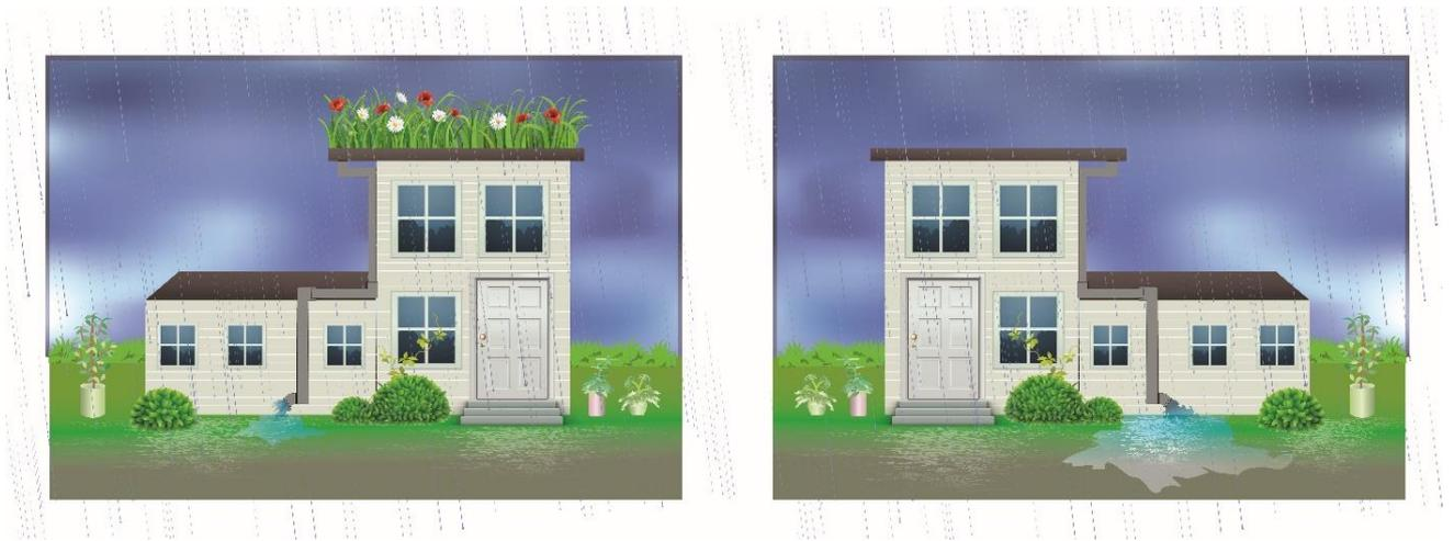
Figure 4-2 - Green roofs help in reducing run-off from heavy rain by retaining water in the substrate and drainage layer
