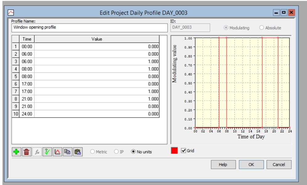
Figure 5-3: Snapshot of window opening profile
