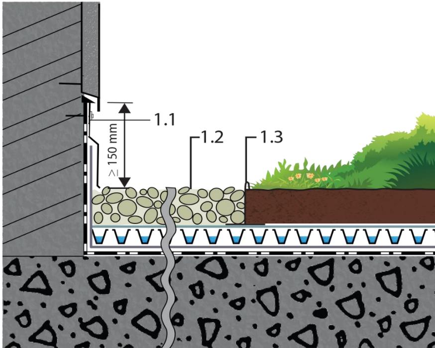
Figure 3-1: Upstand level on building side
