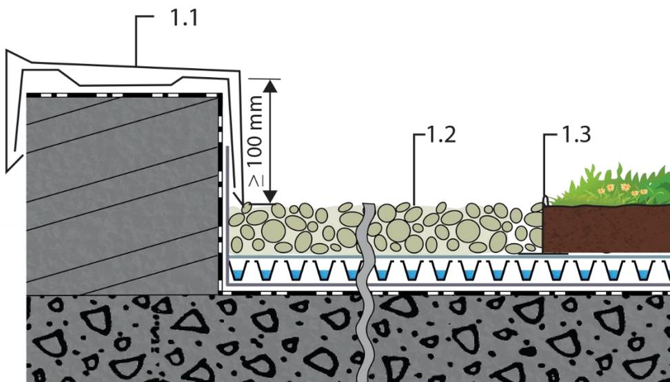
Figure 3-2: Upstand level on parapet wall
