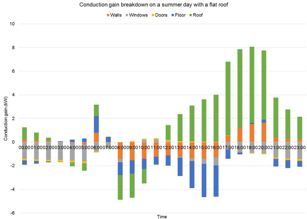
Figure 5-4: Variation of conduction game on a typical summer day for a flat roof
