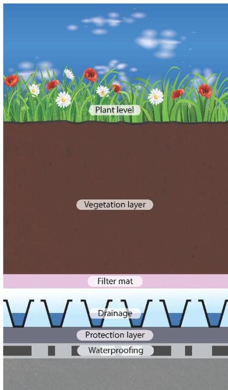
1. Same build up as simple extensive green roof can be used as drainage layer does not need to store much water. The same applies for the substrate layer.
