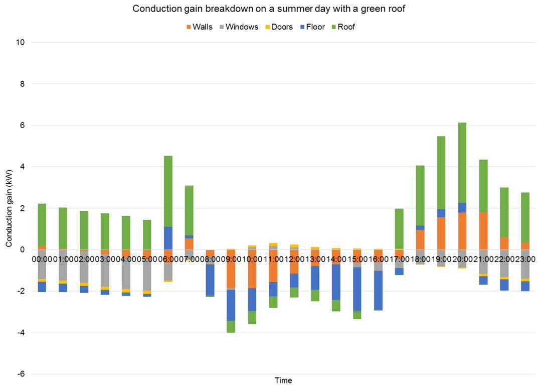
Figure 5-5: Variation of conduction game on a typical summer day for a green roof
