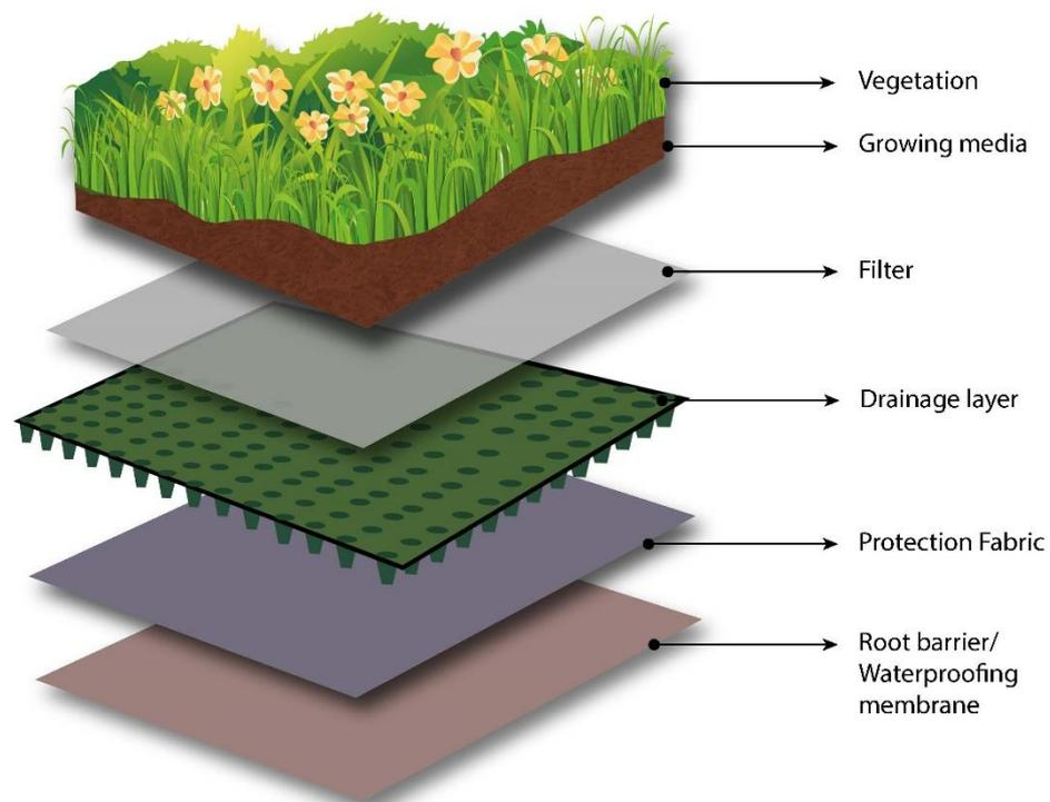
*Figure 2-1: Layers of Green Roof*
