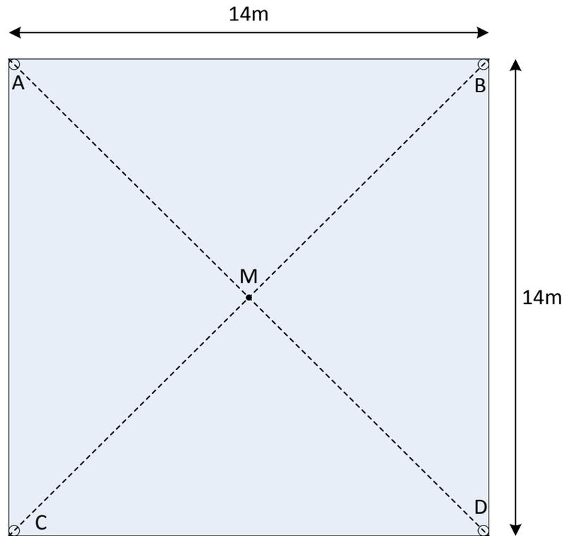
Figure 4-1: Roof example with four 75mm roof outlets at the corners
