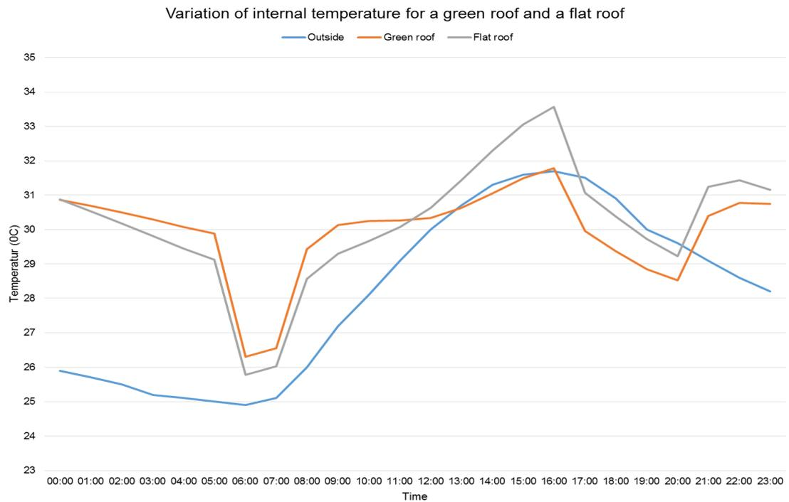
*Figure 5-6: Variation of internal temperature for a flat and green roof*
