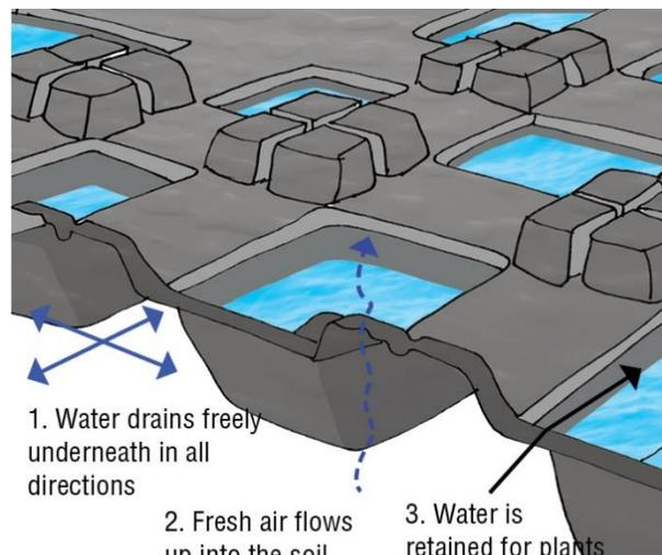
Figure 2-2: Working principles of drainage layer [7]
