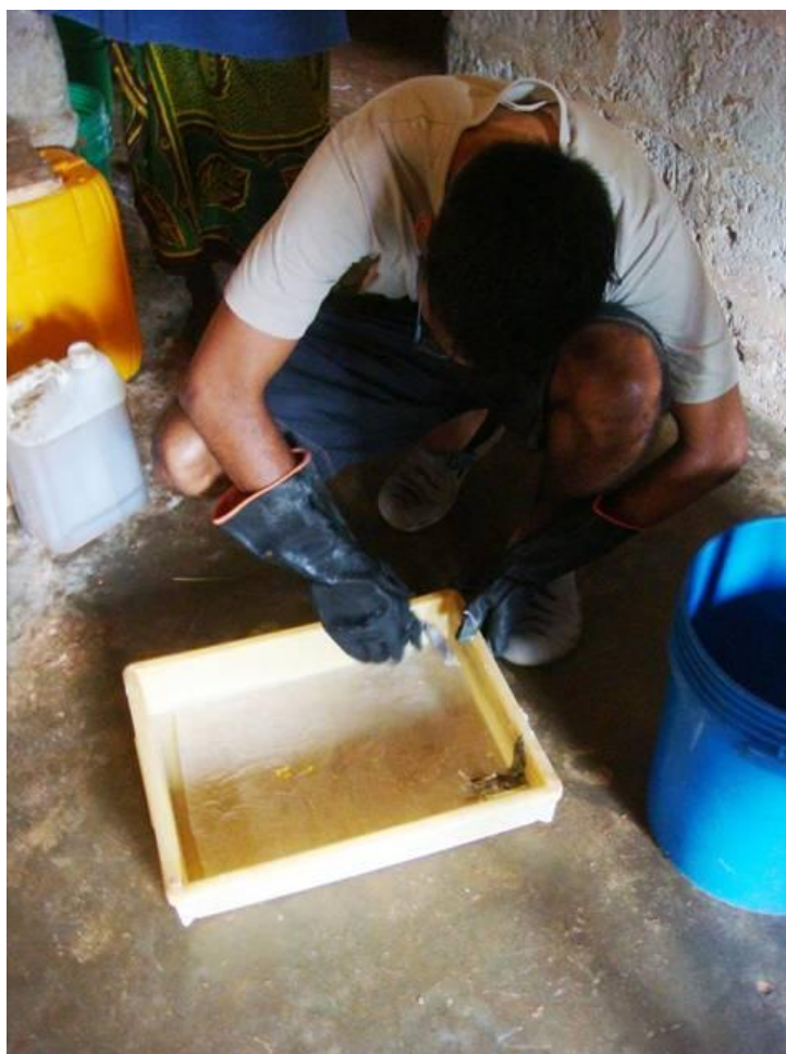
Fig. 33 A trainee preparing a plastic tray (applying Vaseline) for putting the soap mixture
