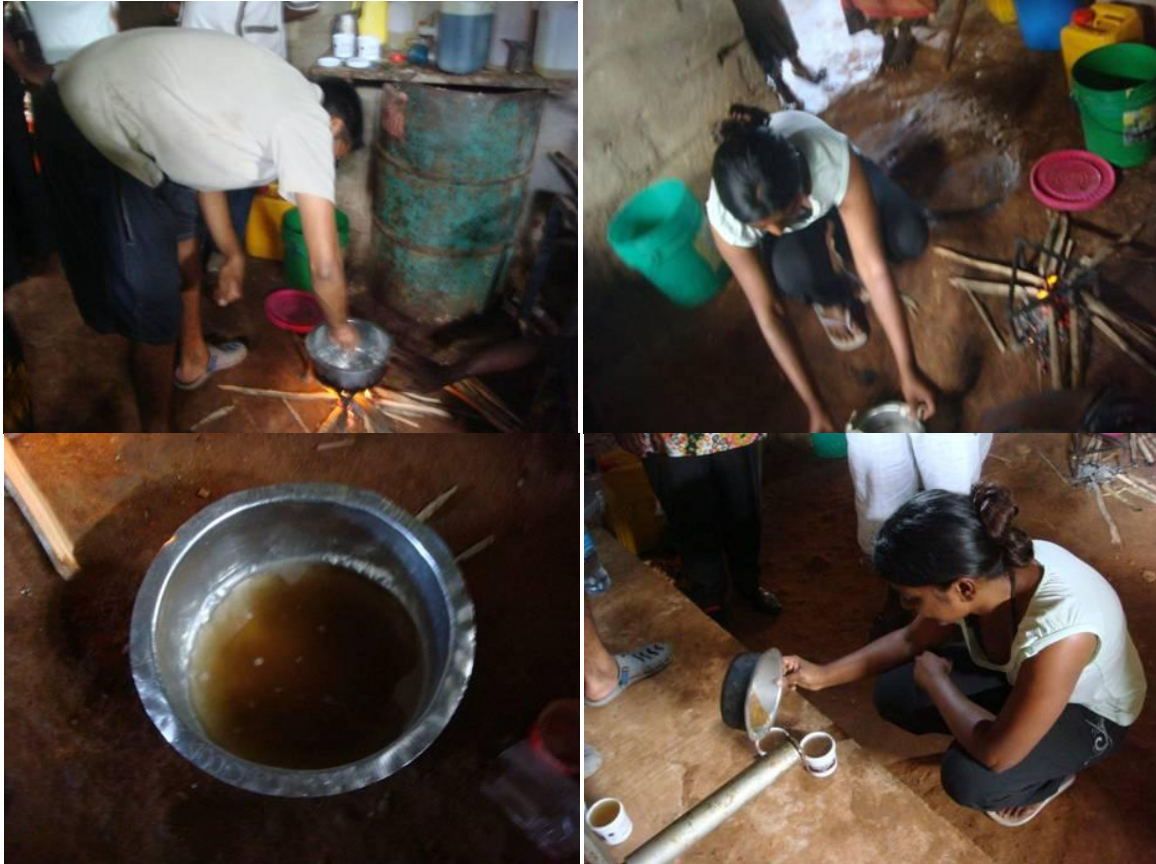
Fig. 38 Trainees making seaweed Vaseline: preparing the fire and cooking pot, adding the Vaseline, mixing, adding seaweed powder, a pot containing seaweed Vaseline, and pouring the Vaseline into containers
