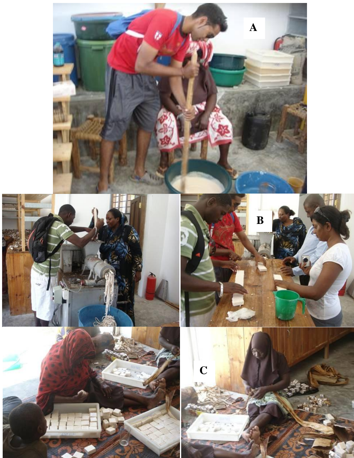
Fig. 27 Making seaweed soap in Paje, East Coast of Zanzibar. A: manual mixing of the ingredients B: making “spaghetti” followed by soap bars by using an extruder C: manual cutting of the soap into pieces and packaging
