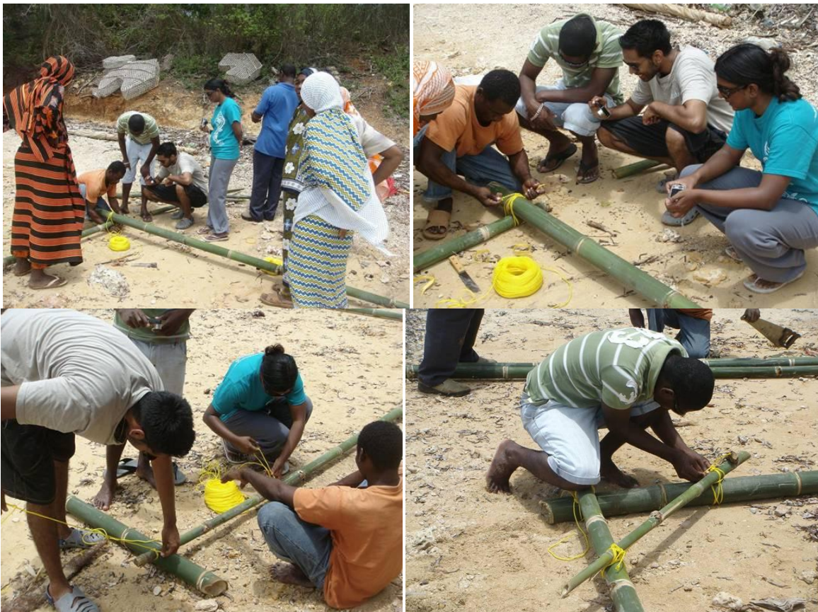
Fig. 18 Trainees tying ropes on bamboo poles to make bamboo rafts. Note also the fixing of a side pole to support the main frame (lower-right photo).
