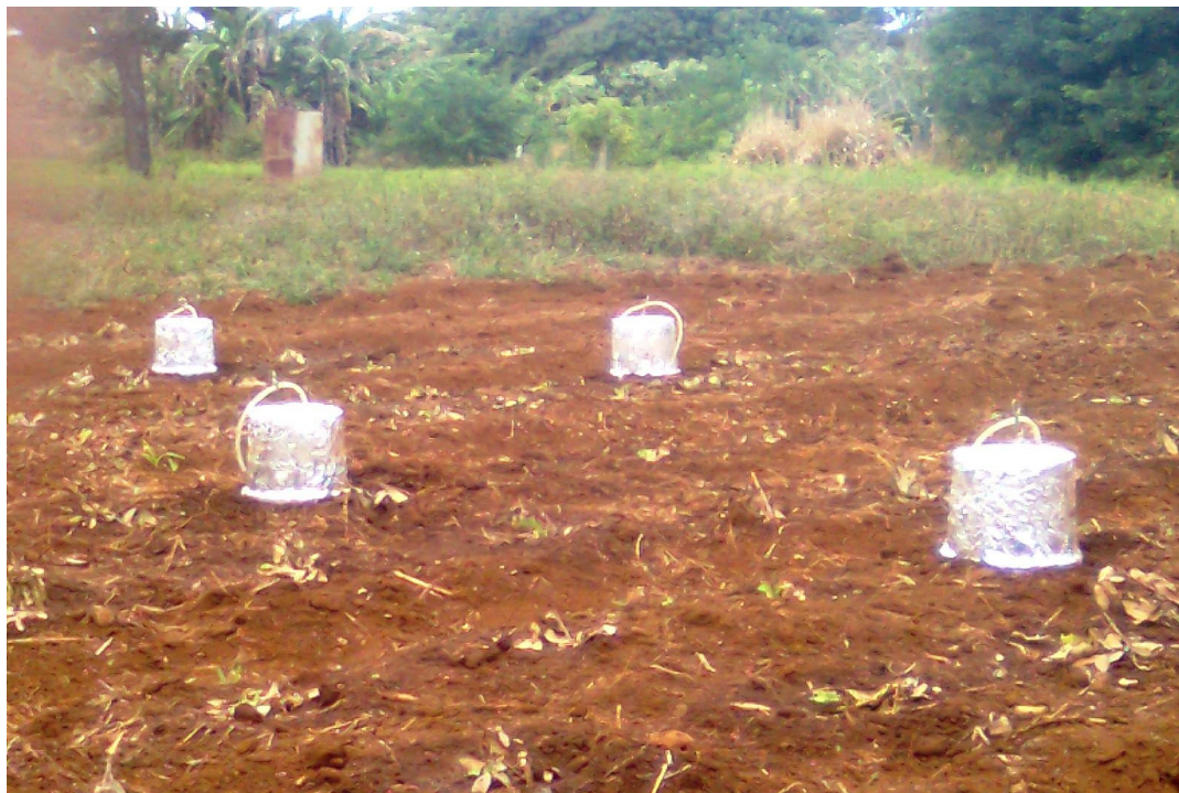
Plate 5: Showing deployment of static flux chambers on the treatments.
