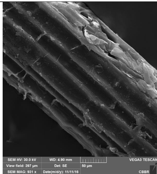
Figure 7.4a: Ravenala untreated fibre at 931X
