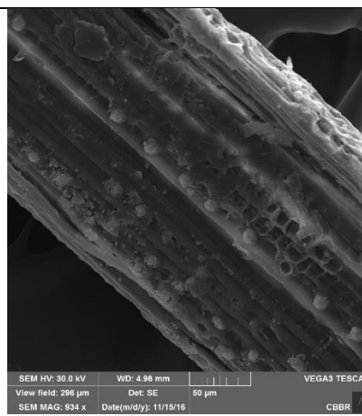
Figure 7.7b: Palmiste Rouge treated fibre at 934X
