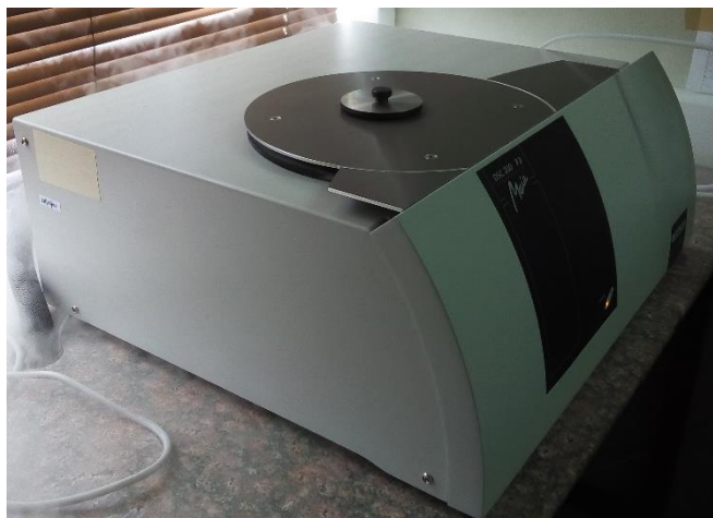
Figure 5.10: Schematic view of the Netzsch DSC 200 F3 Maia® thermal analyzer
