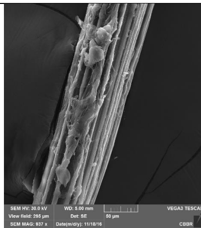
Figure 7.11b: Ananas Bractaetus treated fibre at 933X
