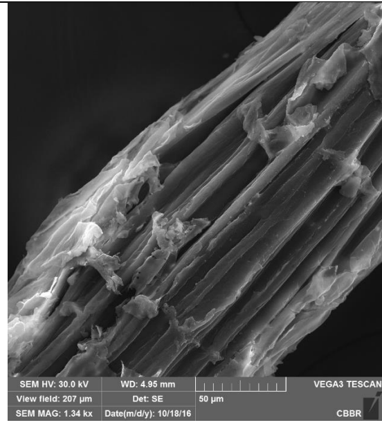
Figure 7.3b: Dracaena floribunda treated fibre at 1340X
