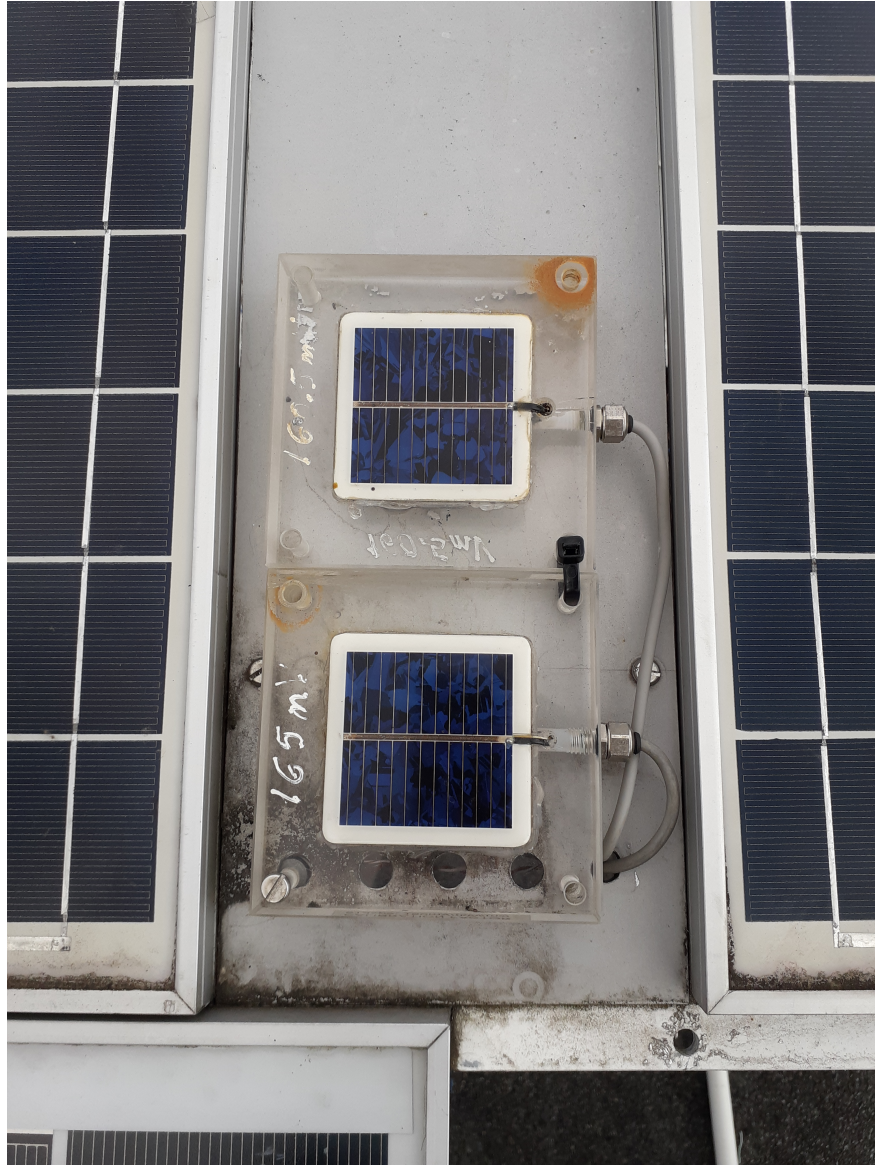
Figure 3.4: Pyranometers in final setup
