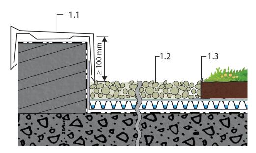
Figure 3-2: Upstand level on parapet wall
