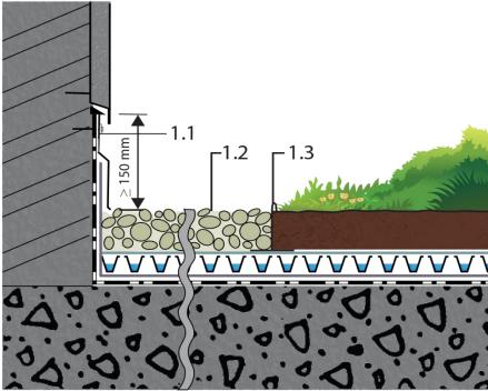
Figure 3-1: Upstand level on building side
