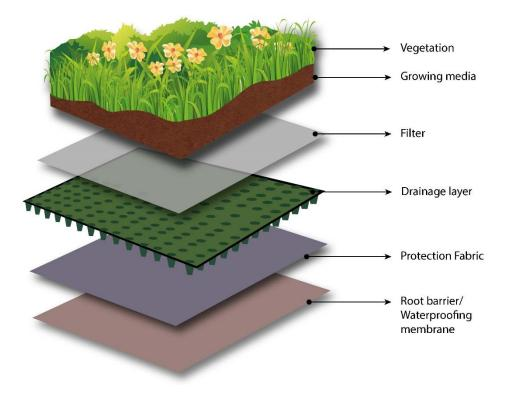
Figure 2-1: Layers of Green Roof
