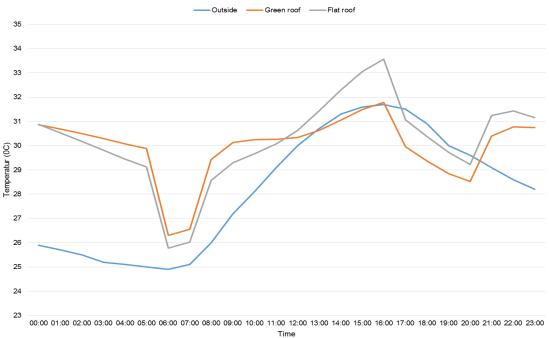
Figure 5-6: Variation of internal temperature for a flat and green roof
