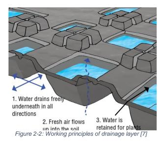
Traditionally, permeable aggregates such as scoria and gravel were used as the drainage layer. This drainage layer was separated from the growing medium by a filter sheet, to prevent blockages. Newer and more modern drainage layers have been designed to [7]:
