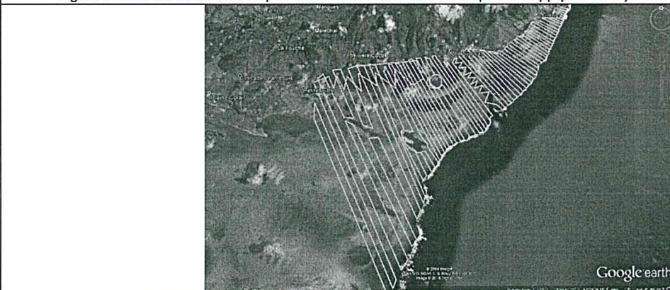
Figure 8: Yellow lines showing transects followed by pirogue during bathymetric survey
