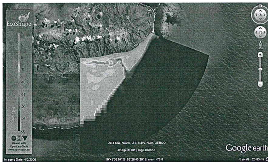
Figure 9: Bathymetry layout used as input to hydrodynamic model
