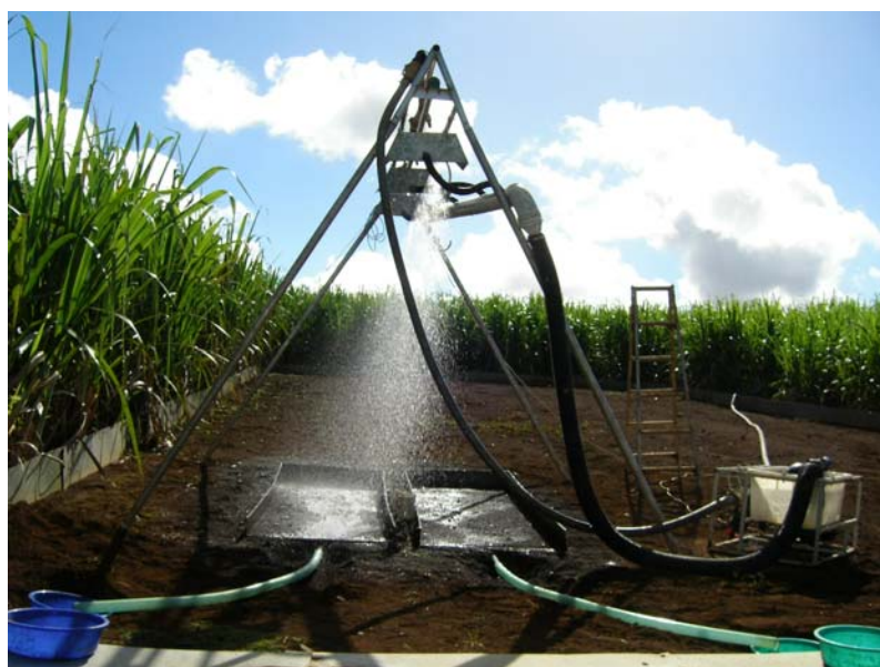
Fig 9. Rainfall simulator used to measure soil loss from bare plot
