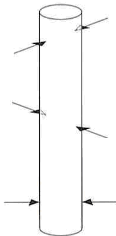
Figure 19: Measuring the diameter of a wire
