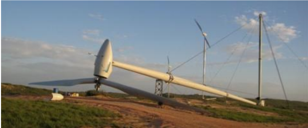
Figure 34: Vergnet 275 kW lay-down model turbines as used on Rodrigues (Clarke 2014) and New Caledonia
