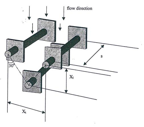
The area of flow found in the equation (1) is the minimum free-flow area of the finned passages i.e. the cross-sectional area perpendicular to flow direction and is given by
