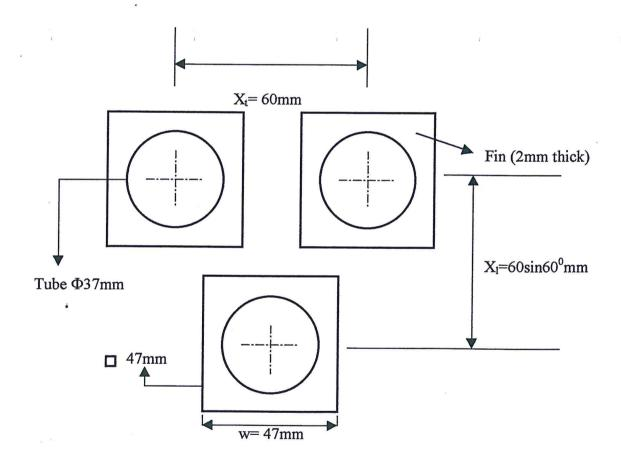
Let s be the distance between adjacent fins and is equal to 12mm. Fin thickness,  $\delta = 2mm$  Tube outside diameter,  $d_o=37mm$  Tube thickness, t=1.5mm
