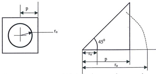
The fictitious radius, r<sub>e</sub> that corresponds to radial fin having the same surface area, as the square and is a function of the dimension p.
